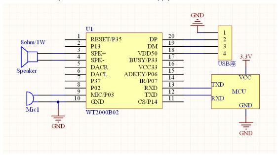
**Note**: WT2000B02 is 3.3 V IO system, direct connect with 3.3V MCU. Connect with 5V MCU need to increase level to convert circuit
