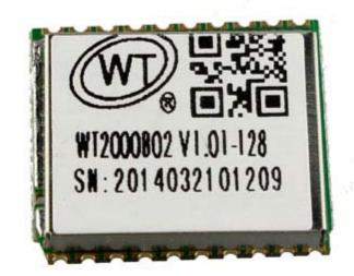
WT2000B02 is MP3 record module, with folder classify, specified file name play and specified index sequence play. According file name to record in specified file or according index sequence to record and play, and specified delete any file in the specified folder.
